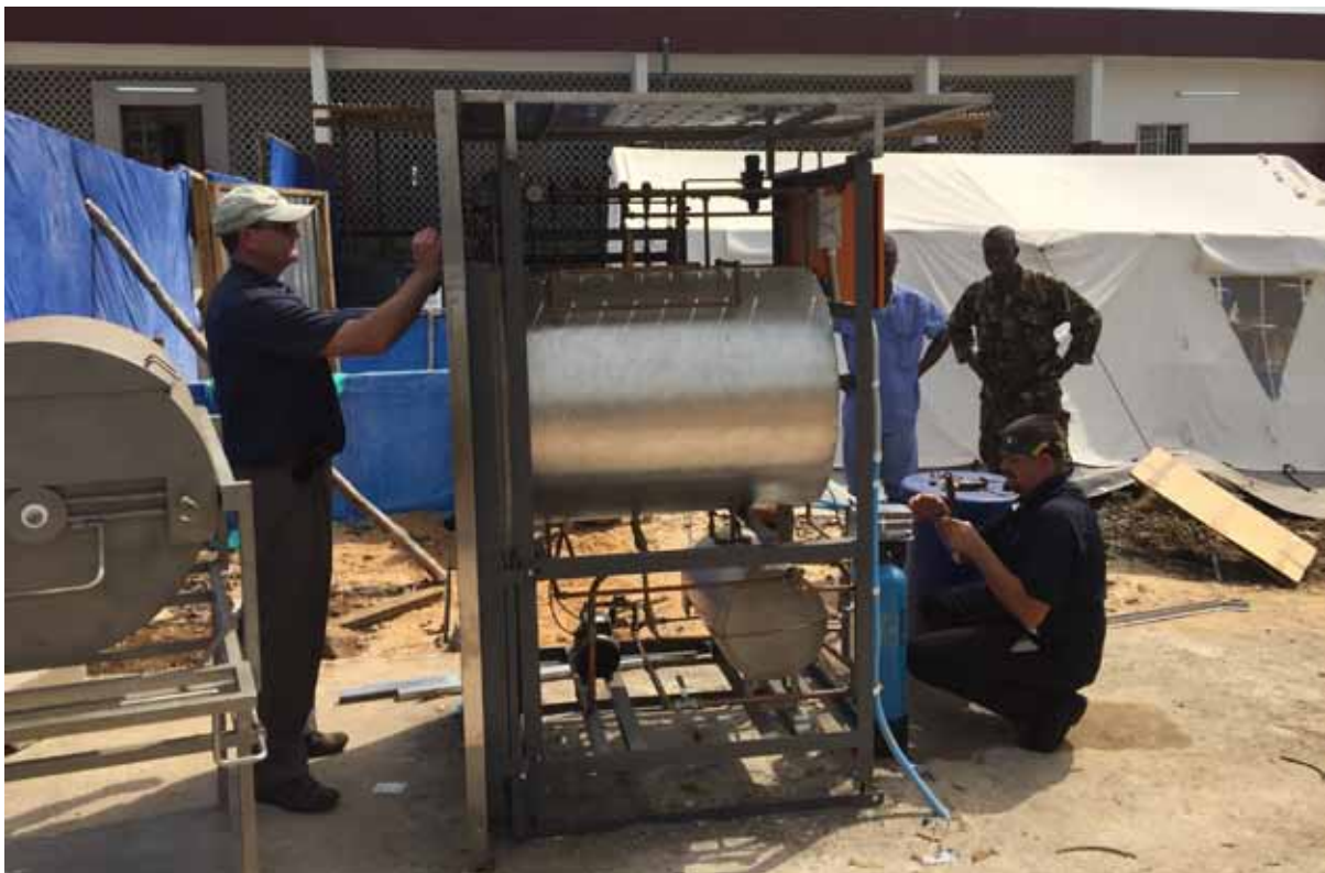
Autoclave being installed in Sierra Leone to treat medical waste. (Photo: UNDP)
