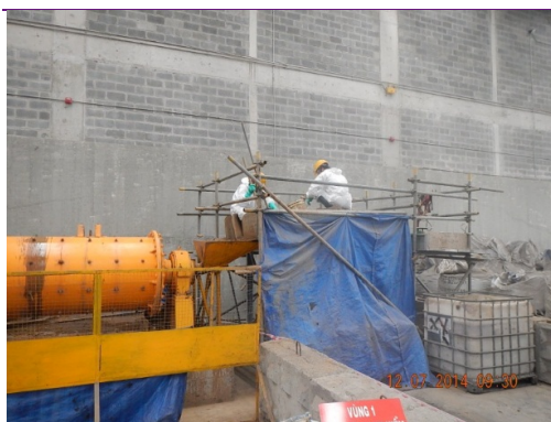
Figure 4.13 Soil was then transferred to a ball mill before adding water to turn it into sludge.
