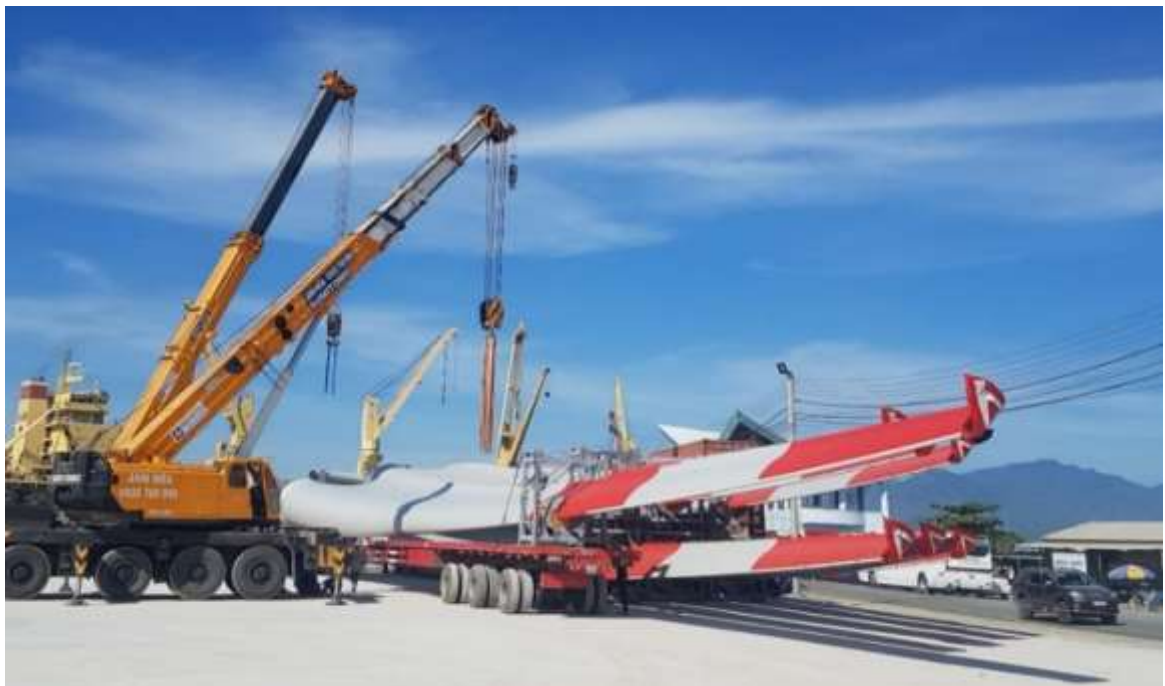
Figure 32. The on-road transportation of a 57 – m turbine blade for Trung Nam - Ninh Thuan Wind power plant 71
