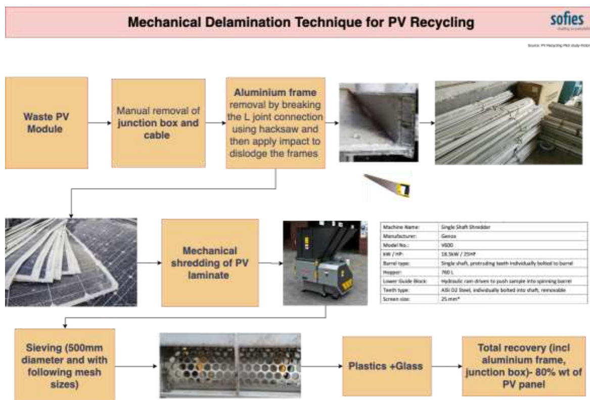
Figure 20. Mechanical delamination of PV panels- Victoria PV Pilot case study 46
