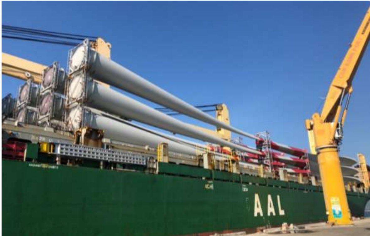
Figure 33. The waterway transportation of a 57 – m turbine blade for Trung Nam Ninh Thuan Wind power plant 72
