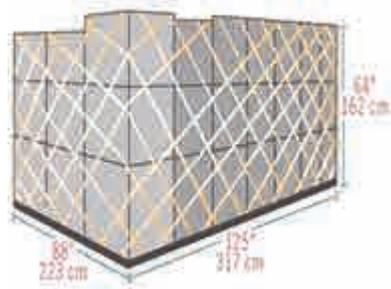
**HALF PALLET****IATA ULD Code:** PLA half pallet with net**Also known as:** PLB, FLA, P9A, P9B, P9P, P9R, P9S**Classification:** HP**Rate Class:** Type 6**Suitable for: Lower deck:** B/47, B777**Main deck:** B707F, B727F, B737F**Maximum volume:** 7.2 cu. m (254 cu. ft)**Maximum gross weight:** 3175 kg (6999 lb)
