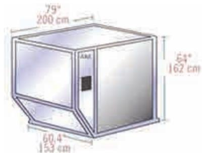
**LD-8****IATA ULD Code:** DQP**Also known as:** ALE, ALN, DLE, DLF, DQP, MQP**Classification:** LD-8**Rate Class:** Type 6A**Suitable for:** B767**Internal volume:** 6.85 cu. m (242 cu. ft)**Maximum gross weight:** 2450 kg (5401 lb)
