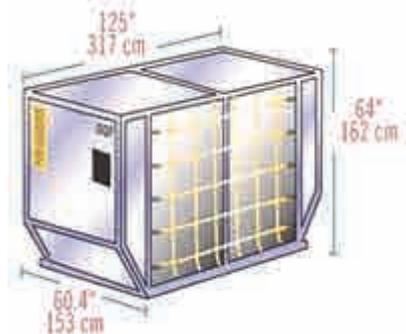
**96" PALLET****IATA ULD Code:** P6P 10ft flat pallet with net**Also known as:** P6A, P6C, P6Q, PMA, PMC, PMP, PQP**Classification:** LD-9**Rate Class:** Type 2BG**Suitable for:** A300, A310, A330, A340, B747, B767, B777, DC-10, MD-11, L1011**Maximum volume:** 21.2 cu.m (747 cu.ft.)**Maximum gross weight:** 6,804 kg (15000 lb)
