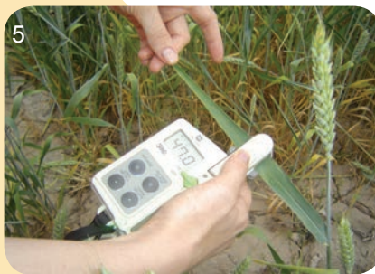
Photo 4. Leaf color chart. Photo 5. Chlorophyll meter SPAD-502. Photo 6. GreenSeeker device
