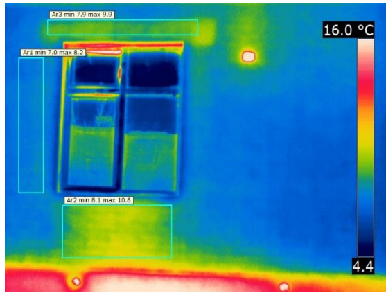
Figure 2.2.6.b) Thermographic image and photo of section of the rear façade of the typical rural house
