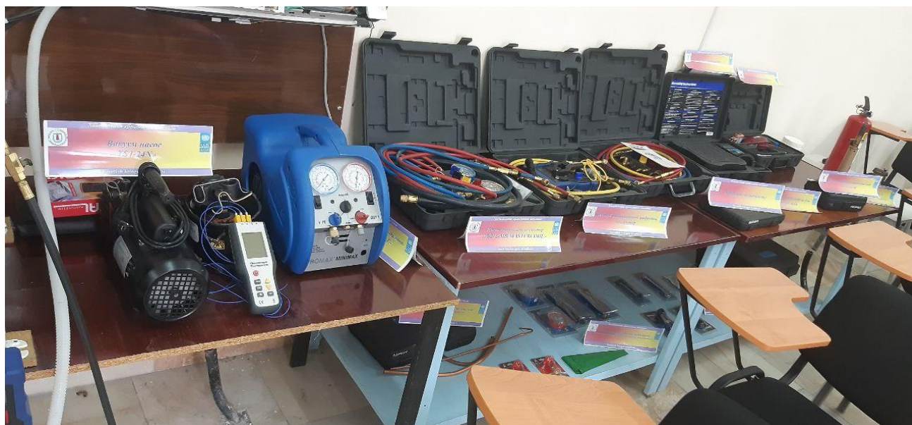
Figure 12. Special tools for servicing refrigeration equipment
