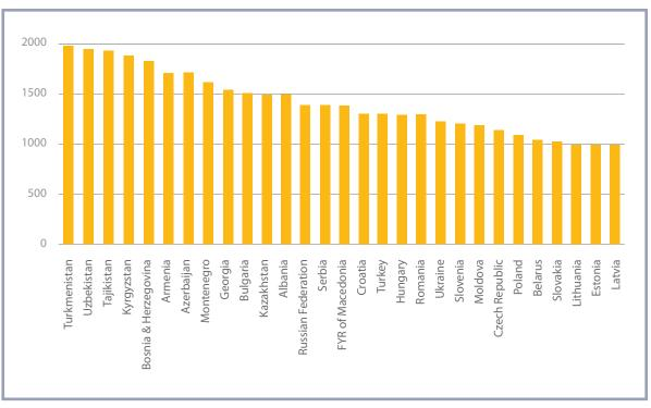
Figure 8: Yearly Average Horizontal Surface Radiation per Country in kW-h/m<sup>2</sup>
