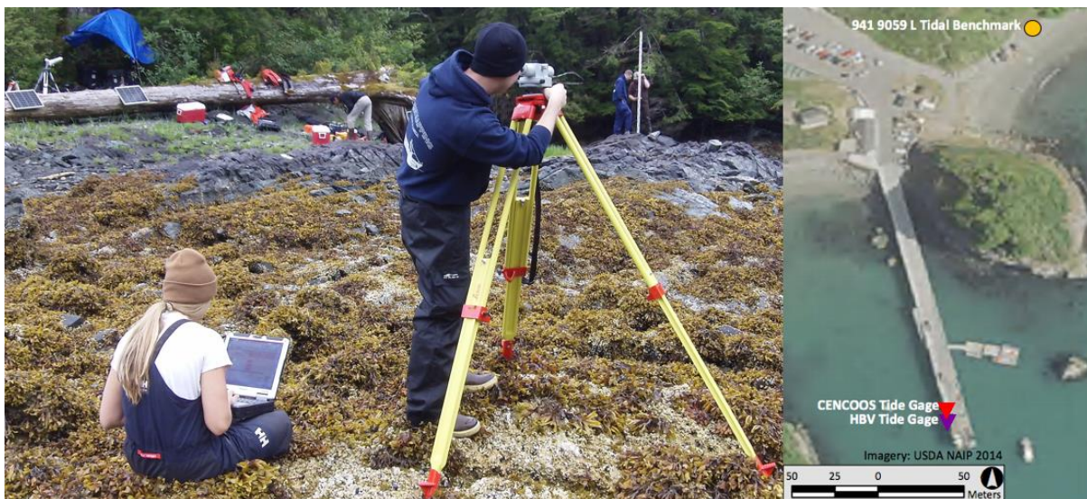
Figure 31. The photo on the left shows a team using levelling equipment to determine the correct position of tide instruments relative to the tide gauge benchmark ( https://noaateacheratsea.blog/tag/fairweather/ ). The image on the right shows the position of two tide instruments (red and purple triangles) and the position of the tide gauge benchmark (yellow filled circle) in Trinidad, California, U.S.A ( http://www.hbv.cascadiageo.org/ )
