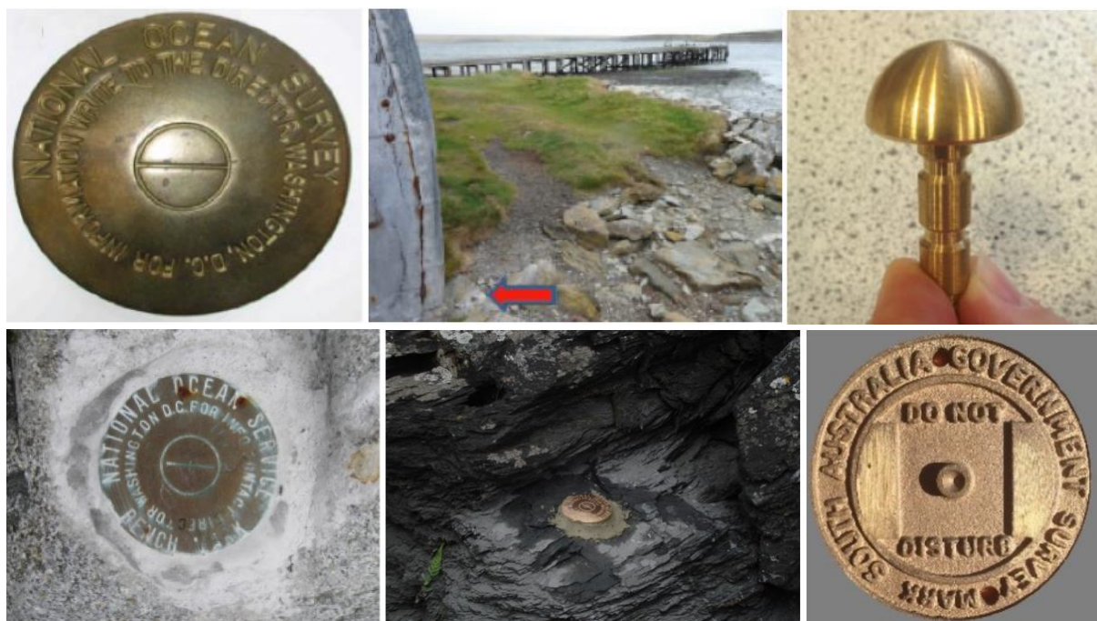
Figure 27. Examples of standard brass benchmarks from different locations around the world (source: OC Manuals and Guides 14, JCOMM Technical Report No. 89, IOC, 2016; https://noaateacheratsea.blog/tag/tide-gauge/ ; https://www.sa.gov.au/__data/assets/image/0016/239101/permanent-survey-mark-brass-plaque.jpg )
