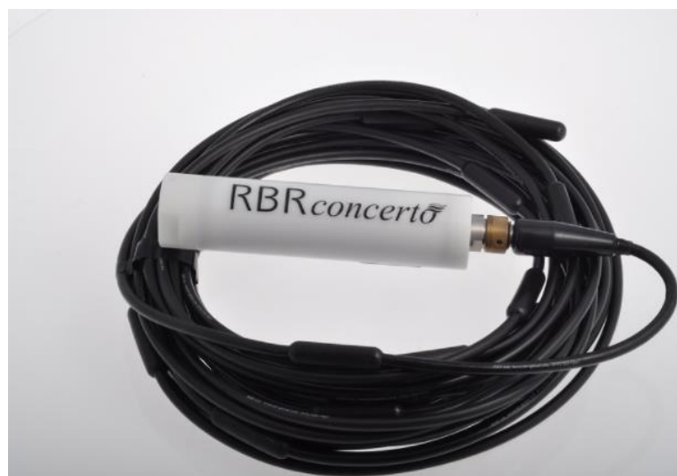
Figure 18. RBR tide gauge and cable to provide power supply and communication. An RBR tide gauge was deployed at Pertamina jetty, Dili, to record water level variations over a 17-day period. The data from this deployment is shown in Figure 3. Typically pressure gauges are cylindrical-shaped instruments. Their lengths range from between 20 and 40 cm, and diameters range from ~2 – 10 cm.
