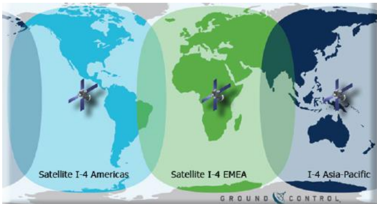
Figure 22. Image depicting satellite coverage for the INMARSAT BGAN system. This satellite system is employed for communication from tide and sea level instruments in Indonesia. (IOC Manuals and Guides 14, JCOMM Technical Report No. 89, 2016)
