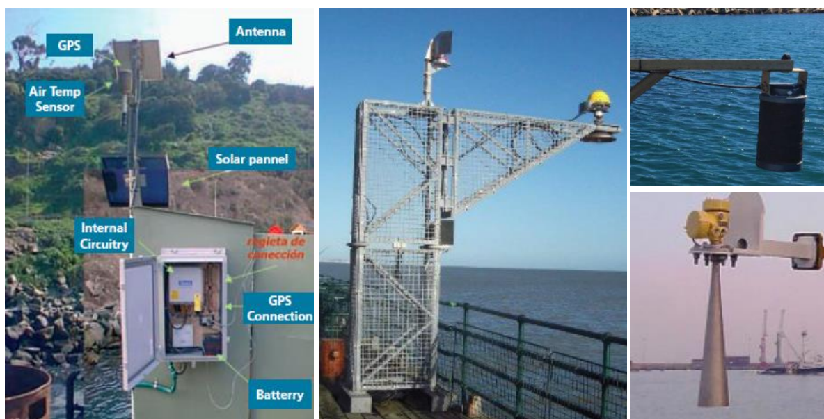
Figure 17. Multiple examples of different radar gauges and radar gauge setups. The first image on the left shows the multi-component setup typically employed for radar tide and sea level observation systems. Three different examples of radar gauges are shown in the central and right images. (IOC Manuals and Guides 14, JCOMM Technical Report No. 89, 2016)
