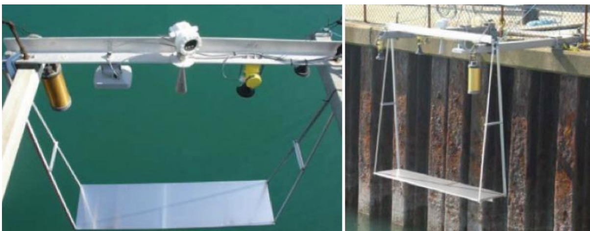
Figure 35. Two images displaying different radar gauges undergoing calibration, using a metal plate to reflect the signal emitted by the gauges at a known distance. (IOC Manuals and Guides 14, JCOMM Technical Report No. 89, IOC, 2016).
