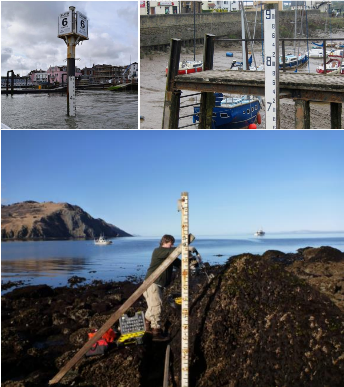
Figure 20. Examples of tide staffs. The top images show tide staffs in the U.K. The top left image is from Cowes Harbour ( http://www.cowesharbourcommission.co.uk/ ) and the top right image is from the Severn Estuary, where tides range over several meters. The bottom image shows a tide staff being installed during a NOAA mission in Kodiak Island Alaska, U.S.A ( https://noateacheratsea.blog/category/2014/page/21/ )
