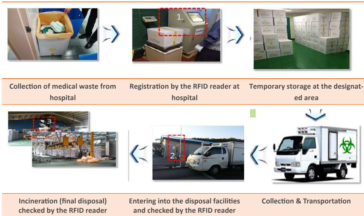
Figure.9 Business procedures about medical waste management system using RFID Technology
