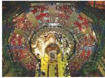
Detector Position Monitoring System: 40 laser systems being installed in CMS at CERN, Geneva
