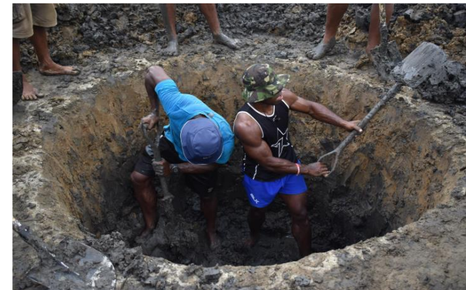
Step 2: The matoji is dug approximately 6 feet and left to be filled with seawater percolating from underground.
