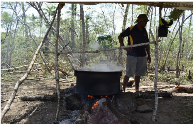
Step 4: The seawater is then boiled in open fire from the dogo (mangrove wood) which is used as fuel.
