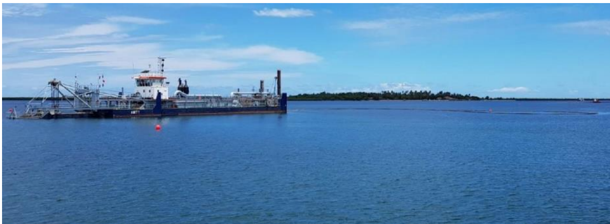
Figure 11: Example of suction dredge with dredge pipe off stern. Source: Fogafale Lagoon Shore Reclamation Preliminary Environmental Assessment
