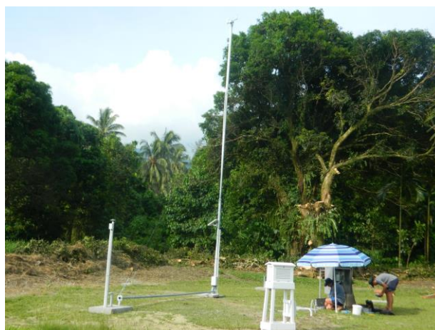
The first automatic weather station installed as part of the SWoCK project at Avuavu in Guadalcanal province.
