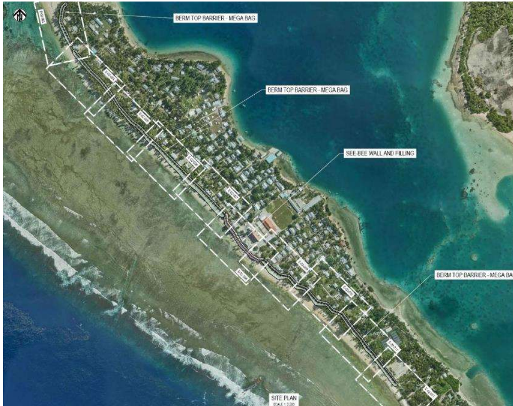
Figure 9: Extent of TCAP coastal protection works on Nanumea
