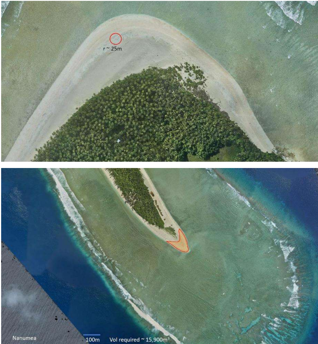
Figure 16: Estimated harvesting surface area for required TCAP sand volumes on Nanumaga (top) and Nanumea (bottom). Areas are calculated using LiDAR data down the reef flat level (2.6m depth for Nanumaga and 2.8m on Nanumea). Source: TCAP Concept Design Report (draft)
