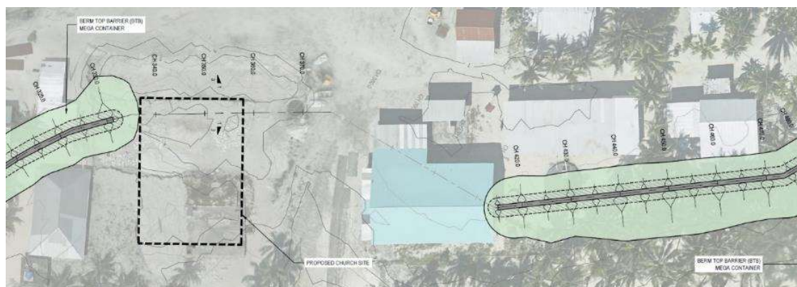
Figure 8: Extent of TCAP BTB stopping the Nanumaga TCS Supermarket (right) and the church foundations (left)
