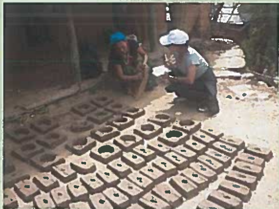
Harkama Pun preparing improved cooking stoves, Pang VDC, Rolpa district
