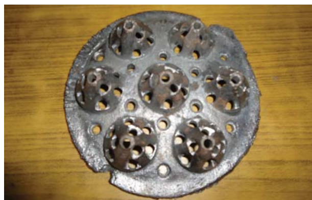
New burner operates without support of fan and adaptor
