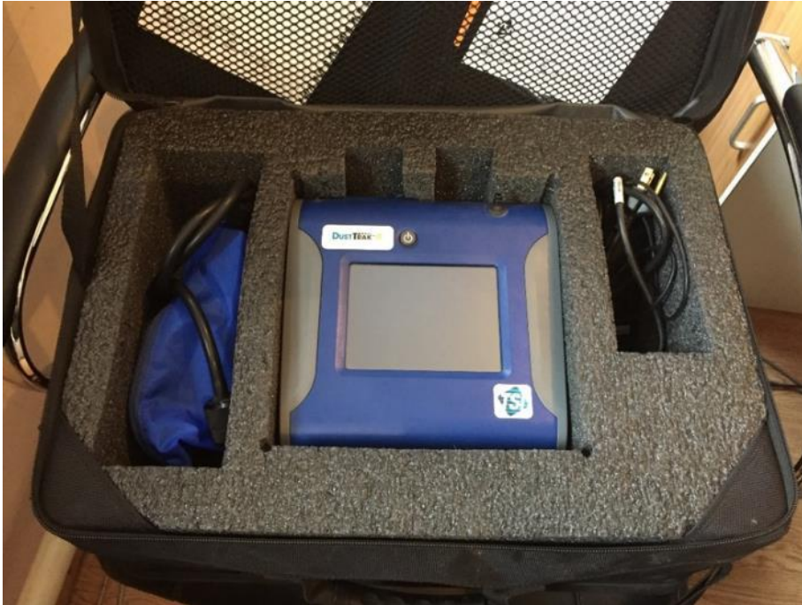
Photo 4. Portable air quality monitoring device DustTrak TSI 8530 used by Tavantolgoi JSC
