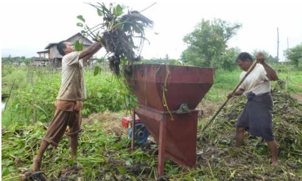
Hyacinth cutter in Kyun Gyi Taung village used for preparing compost
