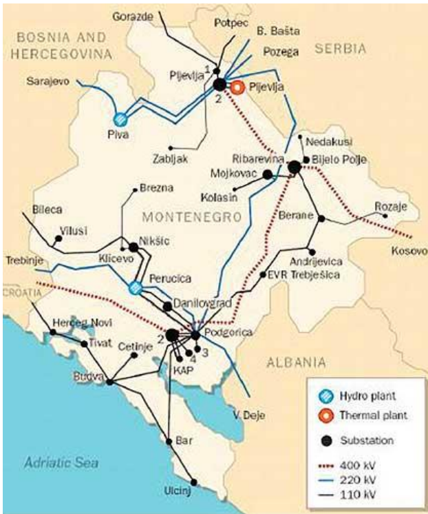
Figure 1: Montenegro Electricity Grid 21
