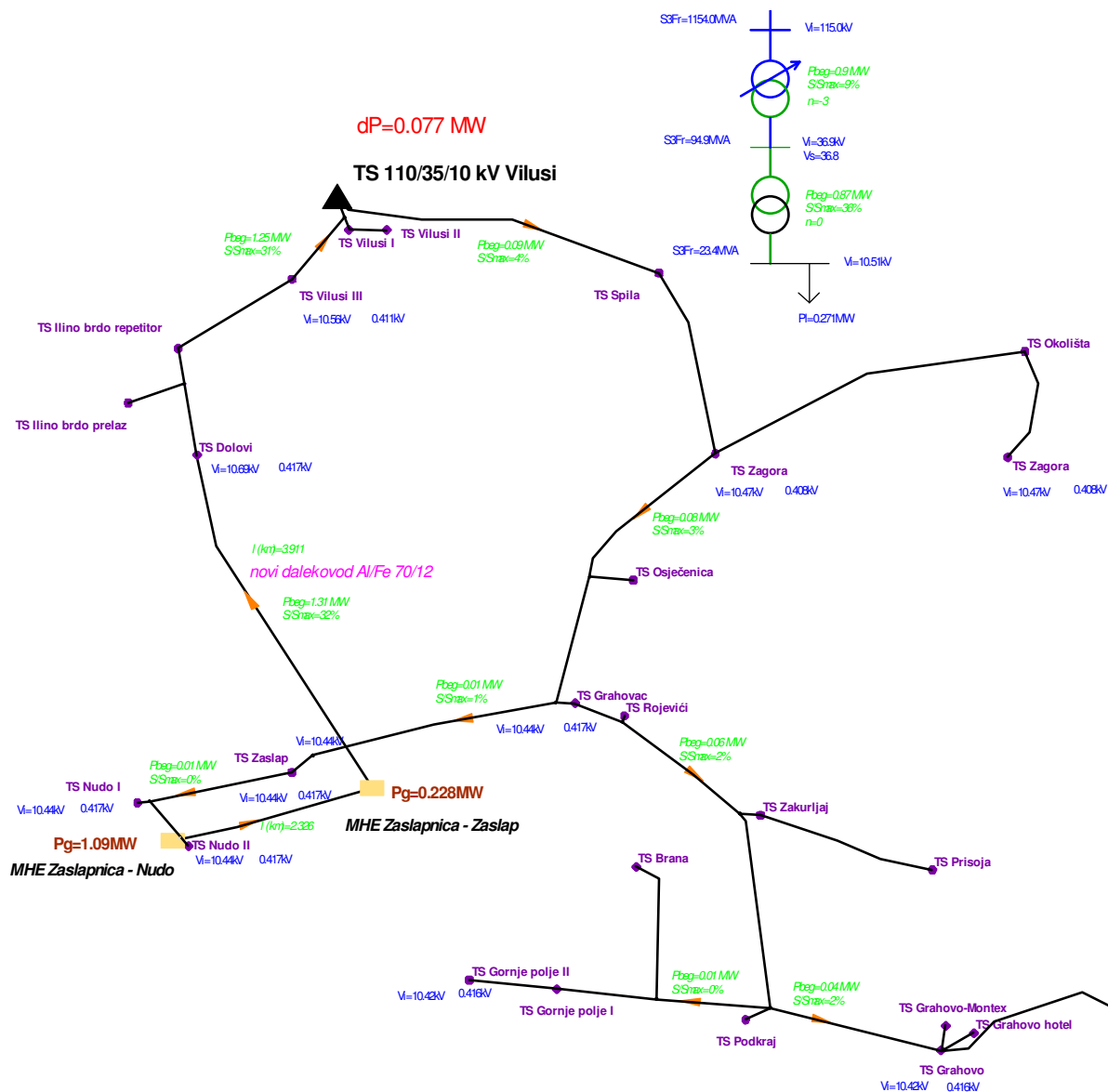
Figure. 22: Analysis results of power conditions – mHE connection to the 10 kV Vilusi feeder with new Al/Fe 70/12 mm 2 transmission line, minimum loads, 2011.
