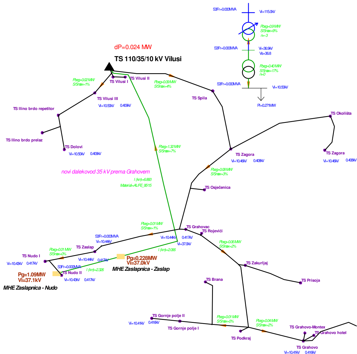
Figure 24: Analysis results of power conditions – mHE connection to the new 35 kV Grahovo feeder, minimum load, 2011
