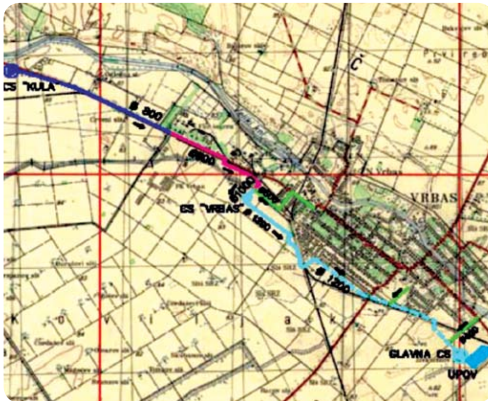
Figure 1 • Wastewater collector phases IV.1, IV.2 and V (Ch. Km 5+999 – km 12+624 and Pumping stations “Kula1” and “Kula 2”)
