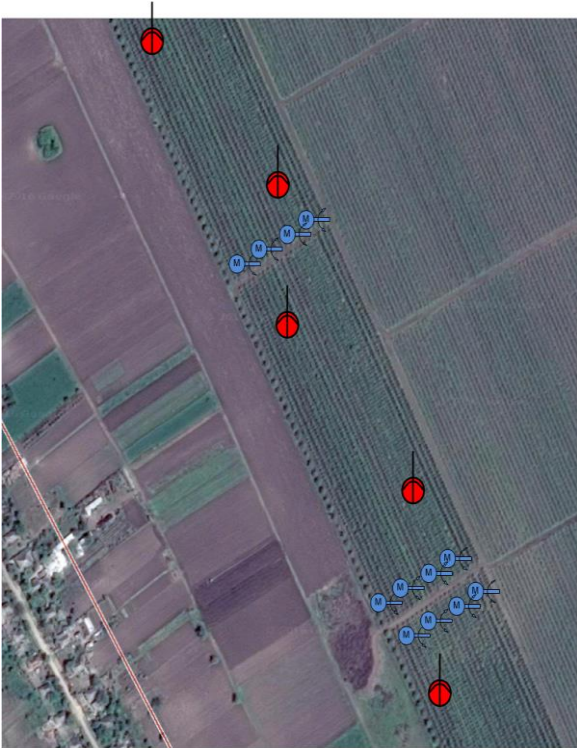
Figure 4. Emplacement map of the integrated sensors module and the valve control module for irrigation system on Fortuna Lapis (Ungheni) farm.
