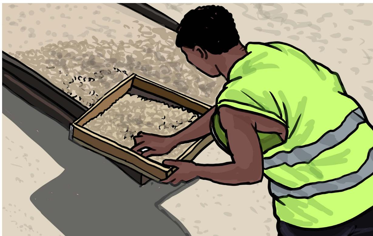
*Figure 14: ASM operator jiggling for Diamond, Tahn, Western Liberia*
