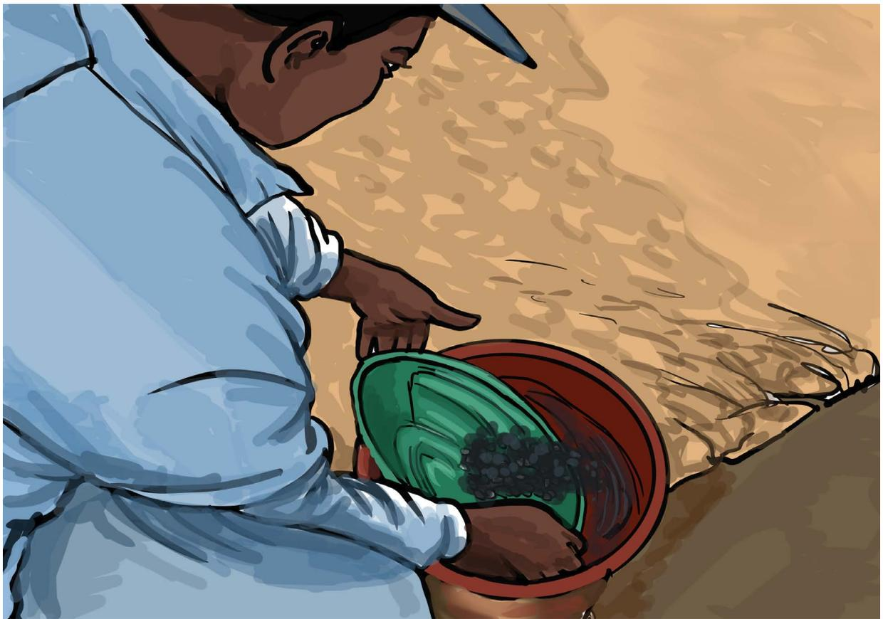
*Figure 17: Plastic pan with ruffles in the side*
