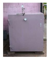
**Figure 16:** Use of Steam Chamber for Soil Sterilization
