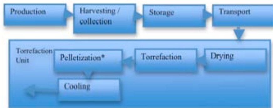
Figure 22: Schematic overview of the feedstock supply chain for torrefaction
