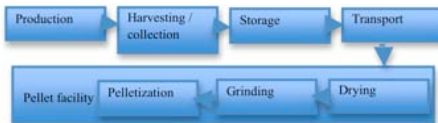
Figure 20: Schematic overview of the pelletisation supply chain
