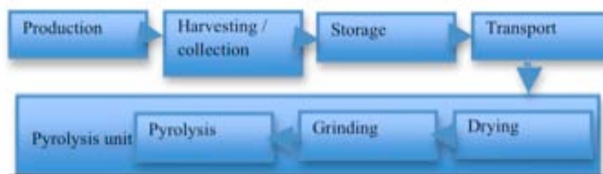
Figure 24: Pyrolysis process steps
