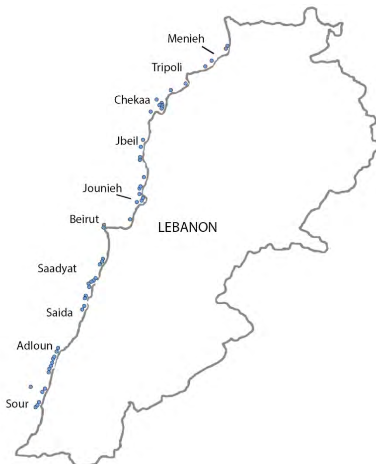
Figure 5-22. Location of submarine springs in Lebanon by means of air borne infrared survey (Shaban, 1999)
