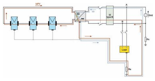
Figure 18 - Current fault example at a plant without galvanic isolation
