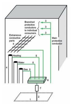
Figure 3 - Components of an earthing system (Source: Schneider Electric)
