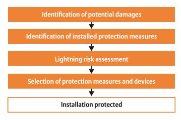
Figure 22 - Steps of the lightning protections assessment process
