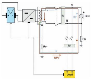
Figure 17 - Current fault example in a floating PV Plant
