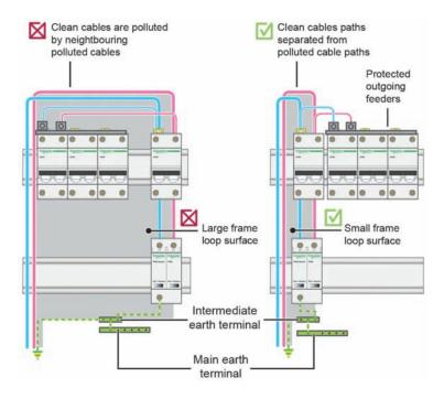
Figure 26 - Recommendation for electric switchboard wiring (Source: Schneider Electric)
