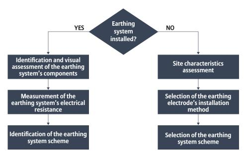
*Figure 13 - Steps of the earthing assessment procedure*
