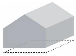
Figure 4 - Buried ring earthing (Source: Schneider Electric)
