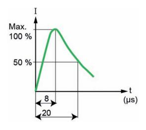
Figure 21 - Indirect strike wave model
