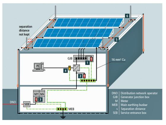
Figure 31 - Case 3: Building with external LPS and insufficient separation distance
