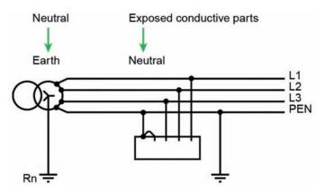
*Figure 9 -* TN-C System (Source: Schneider Electric)
