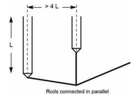
Figure 5 - Earth rods connected in parallel (Source: Schneider Electric)
