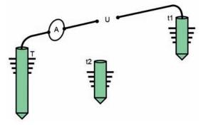
Figure 7 - Measurement of the resistance to earth of the earth electrode of an installation by means of an ammeter (Source: Schneider Electric)
