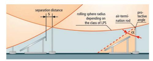
Figure 29 - Rolling sphere method example (Souce: Dehn)
