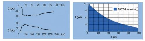
**Figure 19 -** Wave shape and intensities of positive (ground to cloud) and negative (cloud to ground) discharges (left). The measured values for intensity of lightning peak current range from hundreds of amperes to several hundred of kiloamperes (right).
