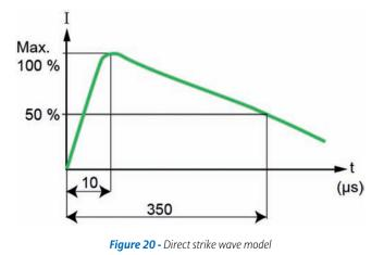
It takes 10  $\mu$ s for the wave to reach 100% of the maximum value The second number is the tail time. The tail time is the time it takes to reach 50% of the value after the wave has reached 100%. Direct lightning tail time: 350  $\mu$ s
