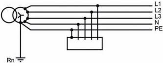
Figure 10 - TN-S System (Source: Schneider Electric)
