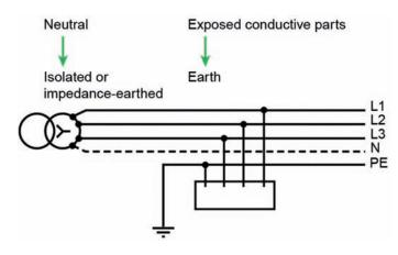
Figure 12 - IT System (Source: Schneider Electric)
