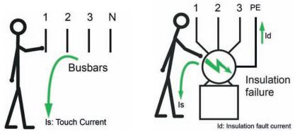
Figure 2 - Direct (left) and indirect (right) contact representations (Source: Schneider Electric)
