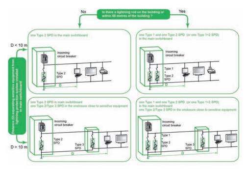
Figure 25 - Proposed process for selecting SPD type (Source: Schneider Electric)
