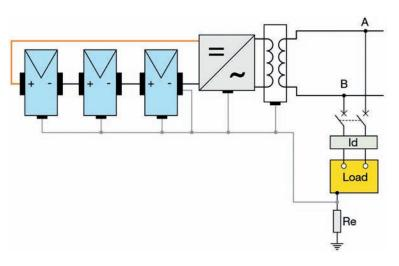
Figure 15 - PV plant with a functionally earthed system
