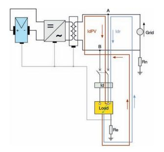
Figure 16 - Exposed conductive parts in a plant with Isolated PV generator on the AC side of the transformer
