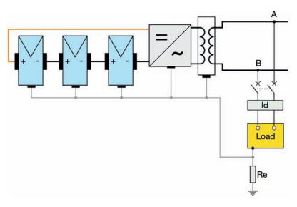
Figure 14 - Plant with isolated PV generator
