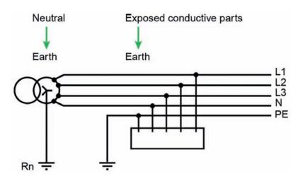
Figure 8 - TT System (Source: Schneider Electric)
