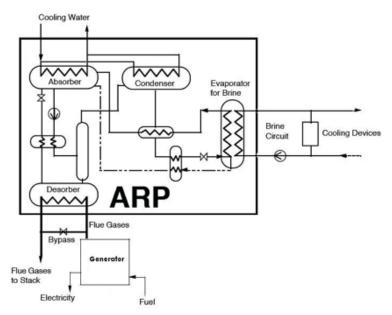
Figure 43: Sample drawing of an ARP on 1,000 kVA generator
