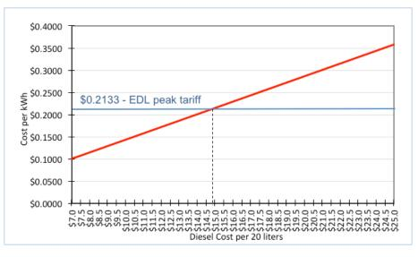
Figure 17: Variation of the generators kWh cost related to diesel cost
