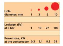
Figure 20: Effect of leakage on power consumption at a system pressure of 7 bar(e).
