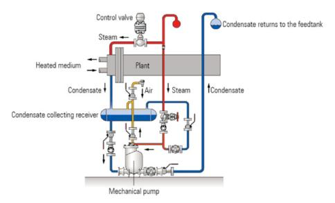
Figure 27: Condensate piping connection (Spirac Sarco 2016)
