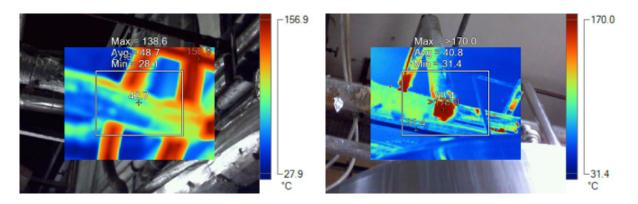
Figure 34: Steam leakage examples
