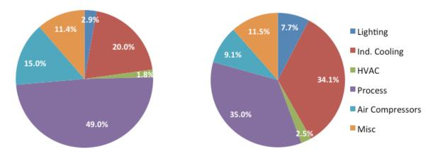
Figure 4: Average electrical load (Left) and energy (right) breakdown for the industries
