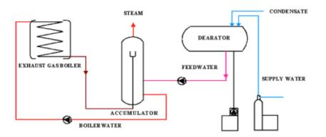
Figure 40: Clayton R System- Operational scheme
