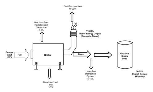
Figure 36: Steam boiler energy balance scheme
