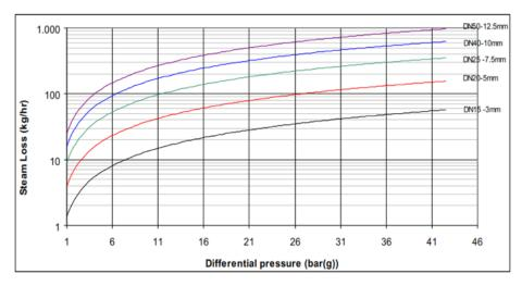
Figure 33: Relationship between steam pressure and steam losses
