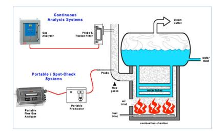
Figure 24: Continuous & portable flue gas and emission analyzers
