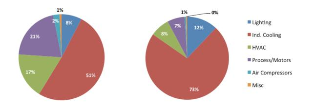
Figure 5: Electrical load (Left) and energy (right) breakdown for the Mixed Use Facility
