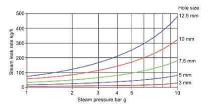
Figure 35: Steam leakage rate as compared to steam pressure
