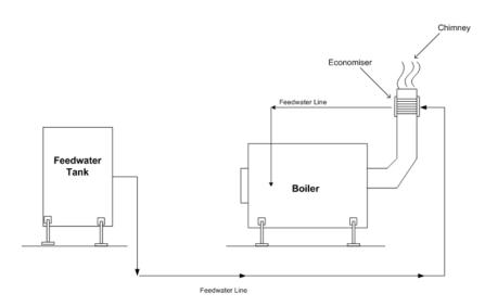
Figure 37: Steam boiler economizer installation
