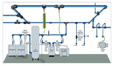
Figure 18: Typical compressed air system components and network
