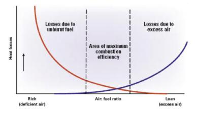
Figure 23: Optimal excess air zone in a combustion process
