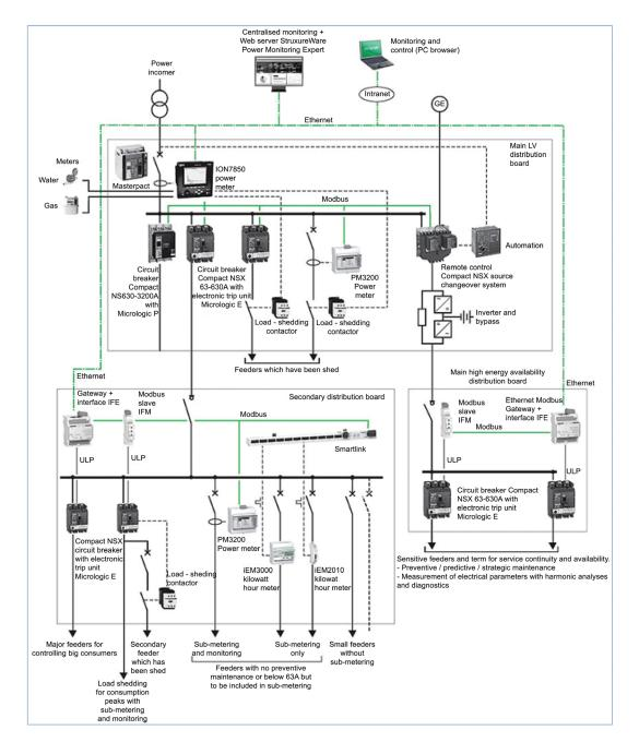
Figure 14: Energy information system architecture (Courtesy: Schneider Electric)
