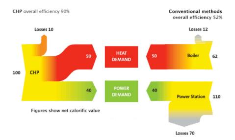
Figure 38: Cogeneration/CHP Energy Diagram v/s conventional systems
