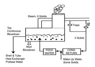
Figure 28: Boiler blowdown system
