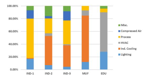
Figure 10: Electrical energy consumption breakdown for the five sites
