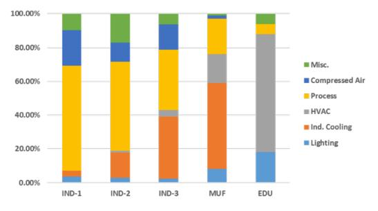
Figure 9: Electrical energy load breakdown for the five sites
