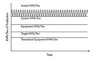
Figure 15: Plant's metering and targeting (The Graph is not zero based and not to scale)
