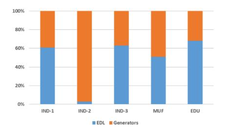
Figure 7: Electrical energy supply by source for the five sites
