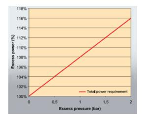
Figure 21: Relation between excess pressure and excess power
