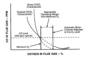
Figure 25: Relationship of CO in flue gas and oxygen level
