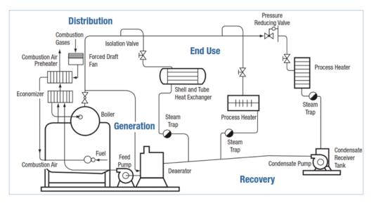
Figure 22: Typical steam network with recovery
