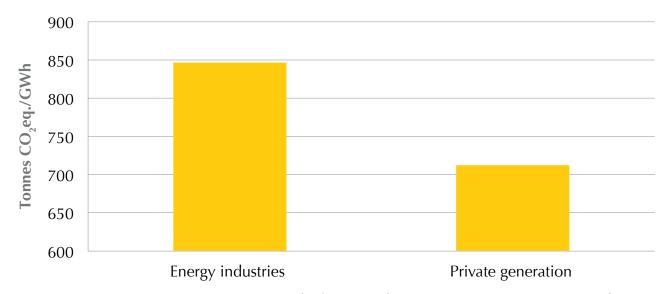
Figure 9: Emission intensity in tonnes CO<sub>2</sub>eq./GWh of energy industries versus private generation in Lebanon
