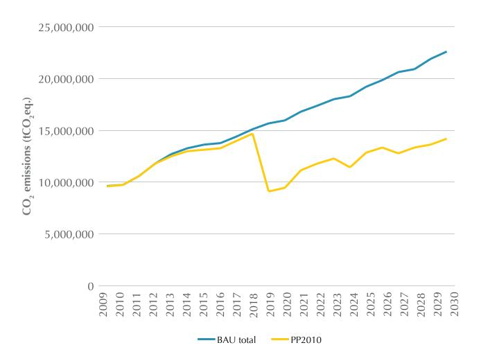
Figure iii: Emission reduction potential from implementing mitigation scenario PP2010
