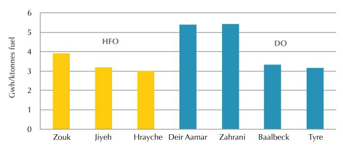
Figure 7: Thermal power plants efficiency
