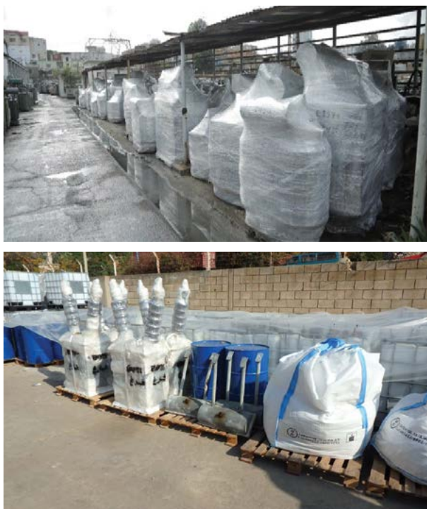
Figure 10-18 Packaged PCB-Contaminated Waste
