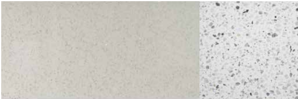
Photo 46 Slabs of reconstituted stone" imported from China (l) and Terrazzo tile from India (r)
