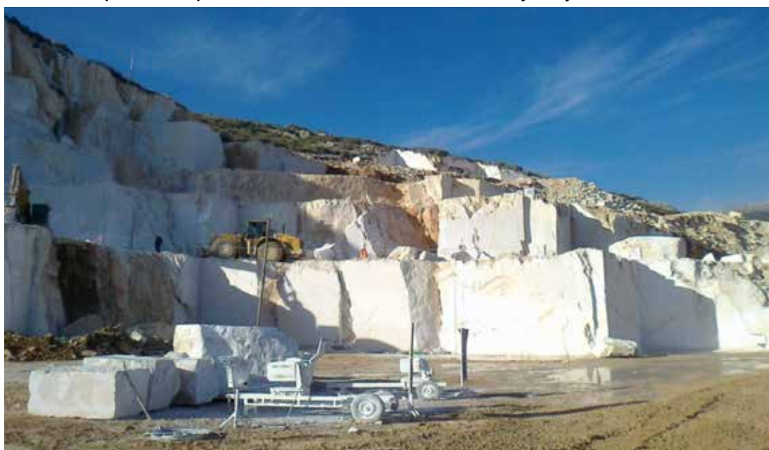
Photo 12 Example of well-planned Dimension Stone Bench Quarry, Italy
