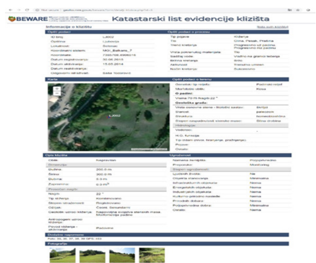
Figure – “aBeware” Android application and filled-in form for Landslide Field Mapping
