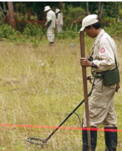
The team use metal detectors to scan the land for bombs and other UXO items.
