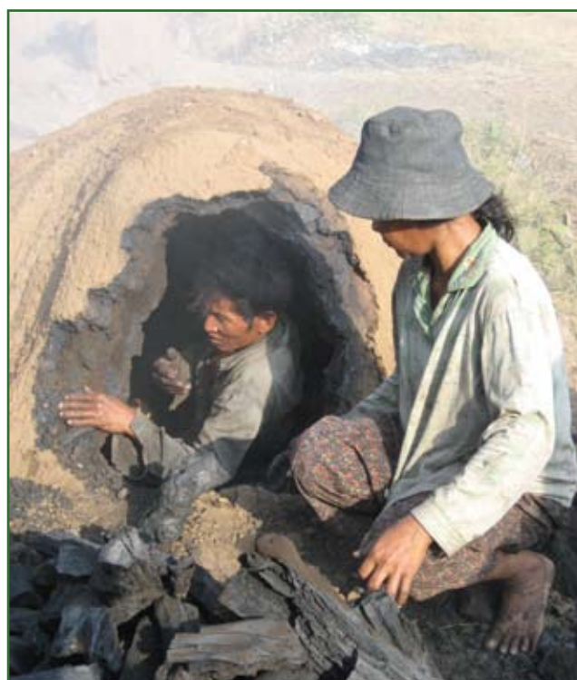
Charcoal production is a thermal process that involves the removal of volatile matter from woody biomass, providing a fuel that is high in pure carbon.
