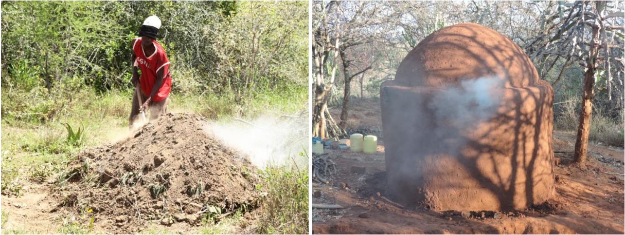
Traditional charcoal burning and a half orange kiln (modern kilns) for sustainable charcoal production at Njiga, Mbeere North
