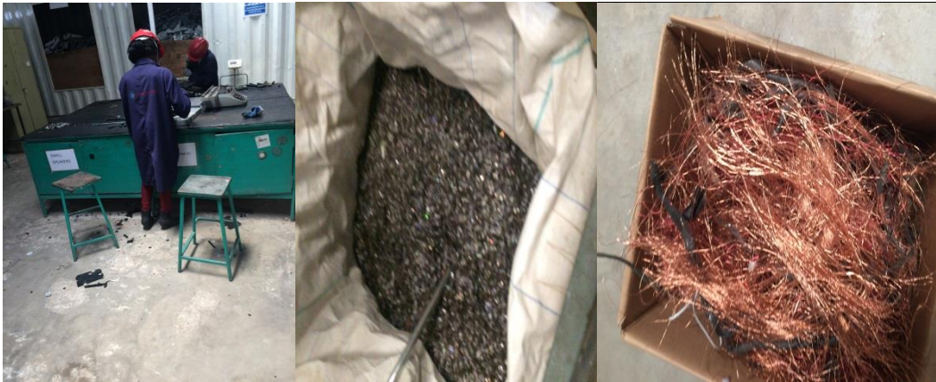
Figure 7.10: E-waste dismantling and some of the products
