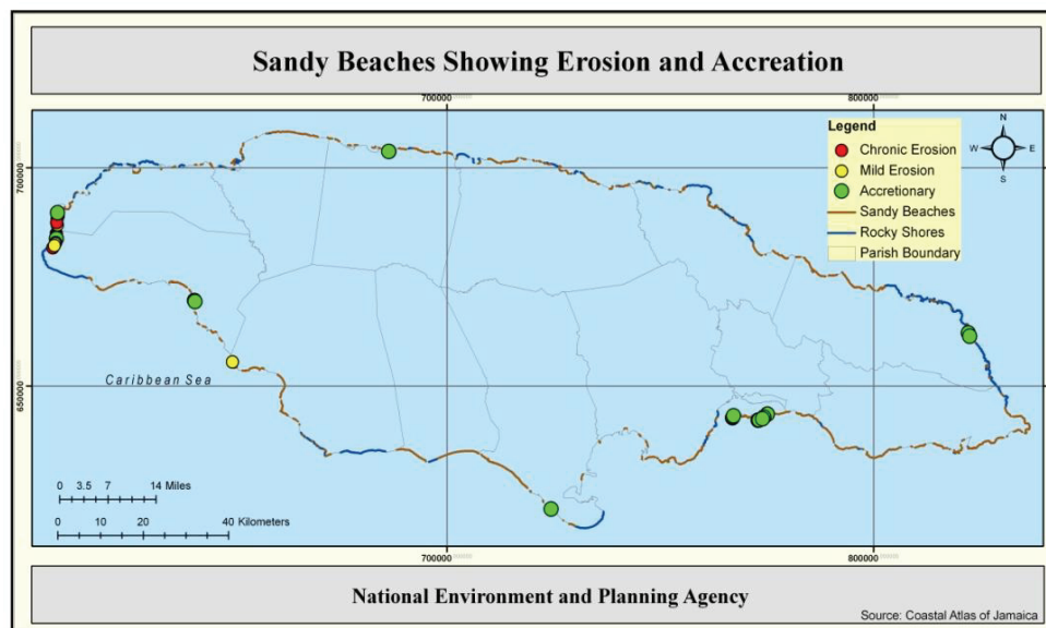
Figure 10: Erosion Trends – Sandy Beaches Showing Erosion and Accretion
