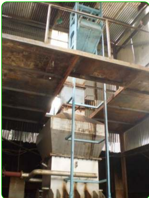
Figure 1 The wood gasifier installed at Glenmorgan tea factory for panning of green tea
