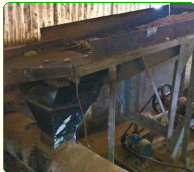
Figure 3 Sifter sifting the heavy/foreign particles
