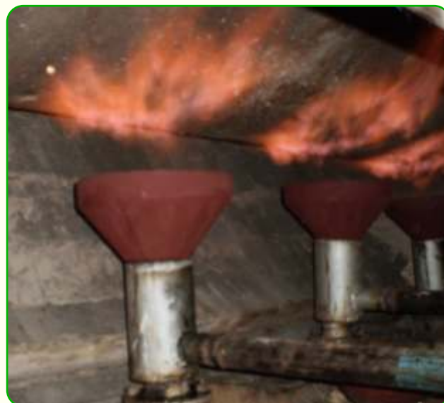
Figure 3 Flames from the gasifier burners provide the required thermal energy
