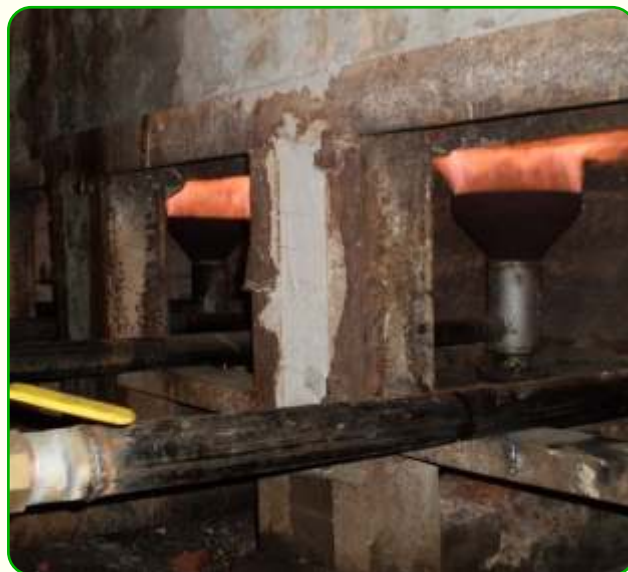
Figure 2 Producer gas produced in the gasifier is transported through the pipes and ignited
