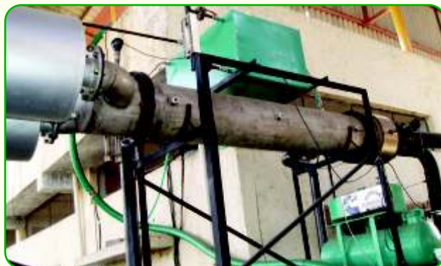
Exhaust cooler specially designed to extract around 80% of the thermal energy from exhaust gas
