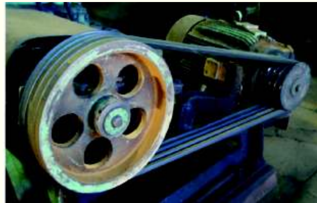
Figure 2: Use of V belts in motors
