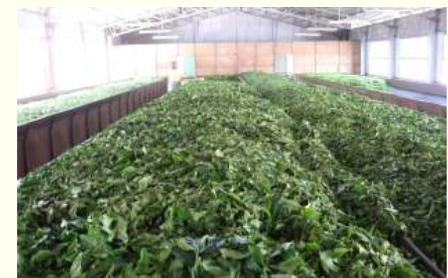
Figure 1: Withering trough loaded with green tea leaves for moisture removal
