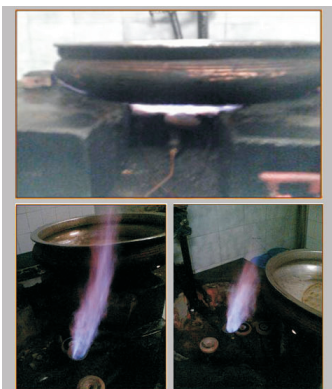
Producer gas replacing LPG in a food industry.
