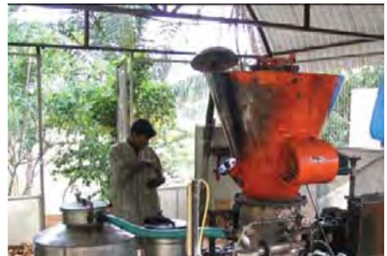
A 9 kW Gasifier system installed for Odanthurai Panchayat water supply system in Tamil Nadu
