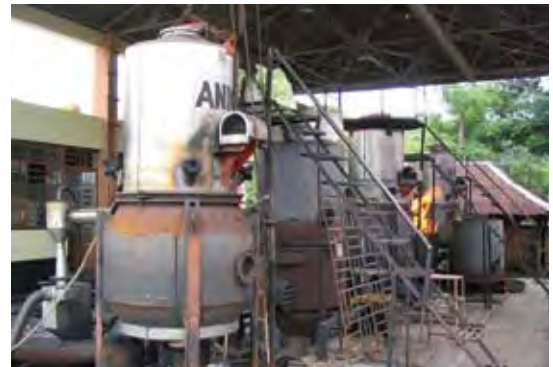
A 5x100 kW Biomass Gasifier at Gosaba Rural Energy Cooperative, West Bengal
