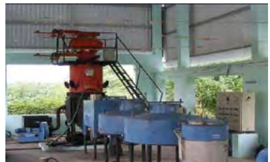
A 40 kW Gasifier installed at Pallipalayam Panchayat in Tamil Nadu
