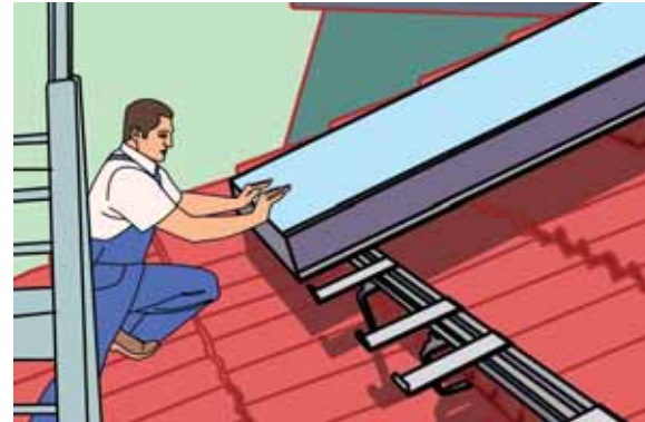
Fig9: Assembly of collector Easy to maintain.
