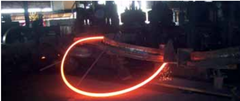
TMT bars in production using producer gas from a biomass-based gasifier plant at Pulkit Steel Rolling Mills, Puducherry
