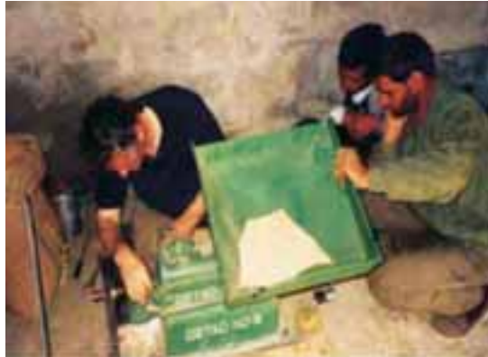
Rice huller being set up
