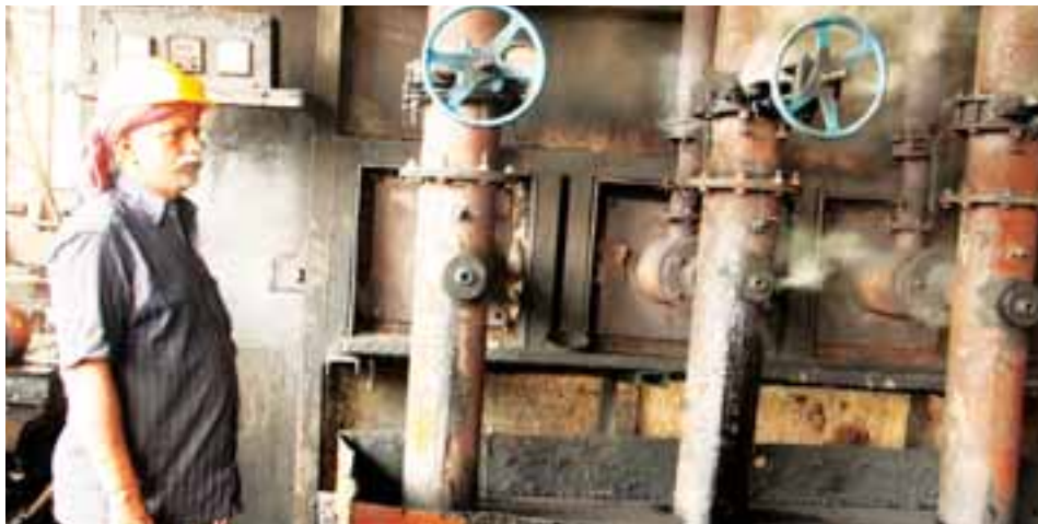
Front view of the energy-efficient re-heating furnace at Pulkit Steel Rolling Mills, Puducherry
