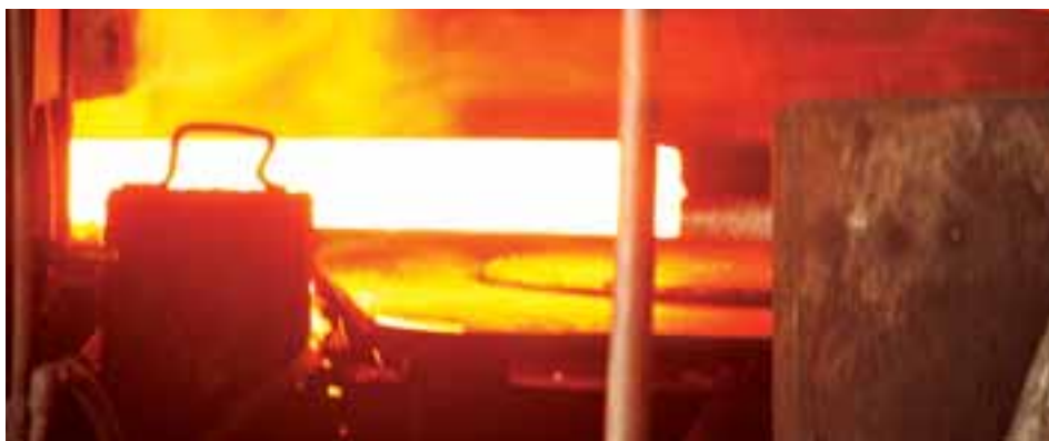
Hot billet after being ejected from the energy-efficient re-heating furnace
