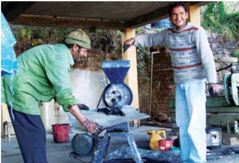
Making fuel briquettes with residual charcoal
