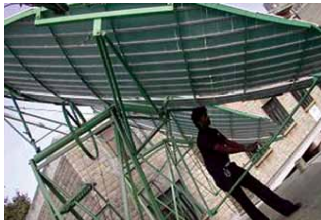
Figure 2: Manual N-S Adjustment Being Done in Scheffler Dish
