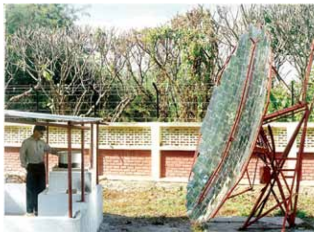
Figure 1: E-W Automatically Tracked Scheffler Dish
