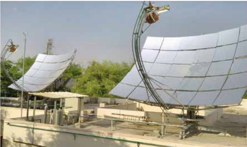
New version of Arun30 dishes at the Police Training Centre for cooking application in Ongole, Andhra Pradesh
