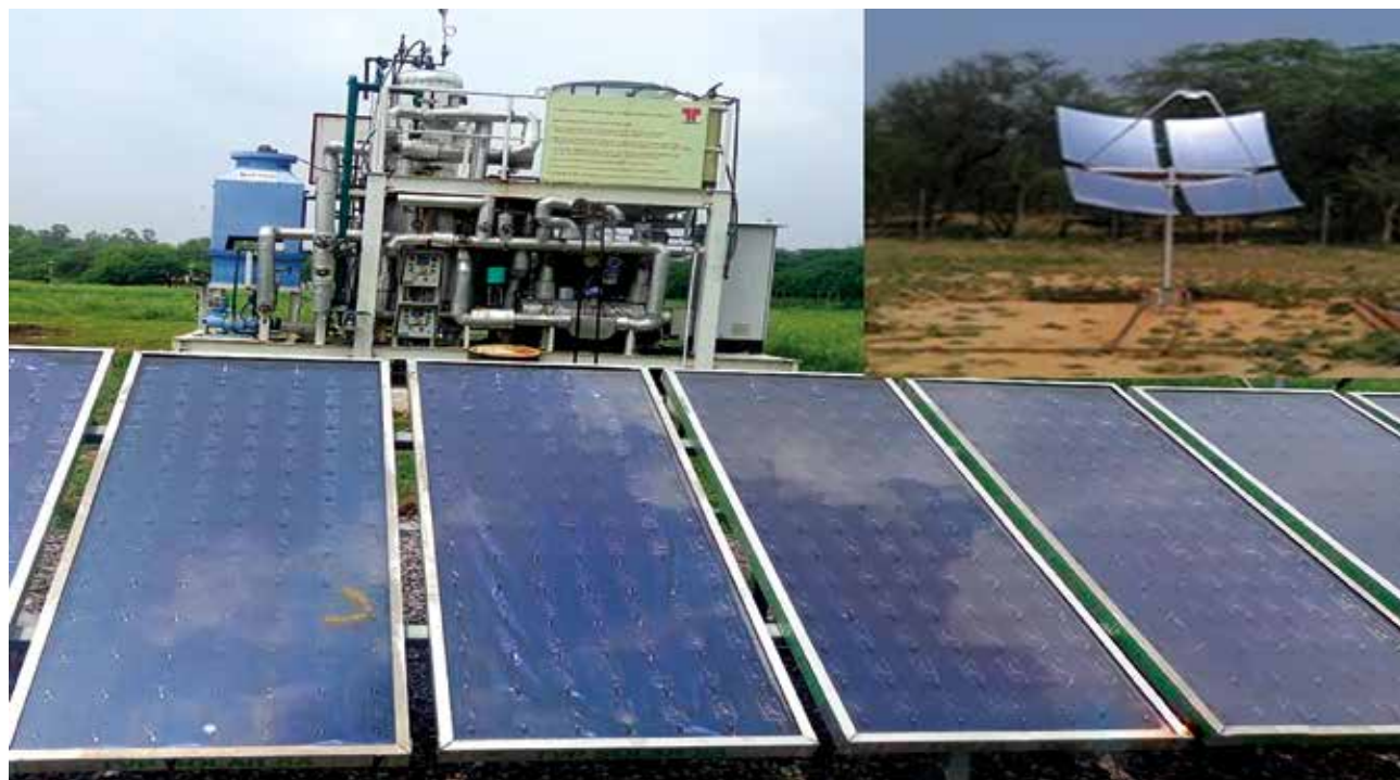
Testing of a CST and evacuated FPC for high temperatures at NISE
