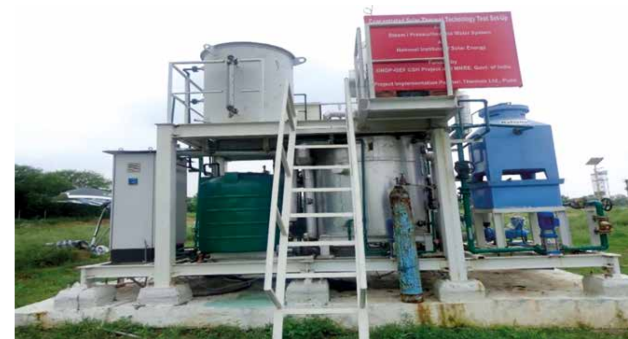
Hot water/steam based test set-up for CSTs at NISE
