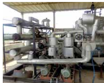
Thermic fluid based test set-up for CSTs at NISE
