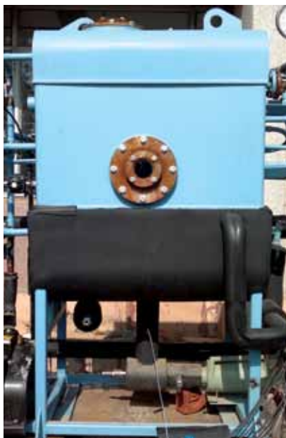
Non-imaging concentrators coupled to Solid Adsorption Based Machine (5 kW Cooling Capacity)
