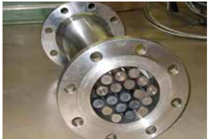
Image 1: Cylindrical capsules filled with PCM integrated into a pressure vessel
